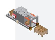
At this stage, the printed decor paper receives an application of a melaminic resin by an immersion process. Thanks to our comprehensive technological expertise, our customers are able to achieve an ultra-robust surface finish for furniture, countertops, interior fittings and floors.
